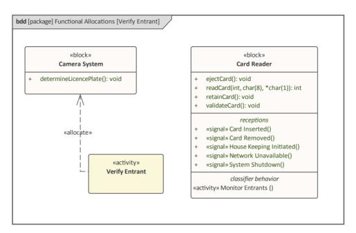
In this diagram the engineer has created two functional allocation relationships that describe how the work specified in the Activity *Verify Entrant* will be carried out. One relationship targets the Camera System that is used to capture the vehicle's licence plate in order to determine if the particular vehicle has been authorized for entry. The other relationship targets the Card Reader Block that is used to determine that the card owner has a relationship with the Parking Station.
