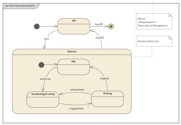
The message in the Sequence diagram Start Vehicle is the trigger that will cause the vehicle to transition from the Off state to the Operate (on) state. Enterprise Architect allows these transitions to be defined in detail.
