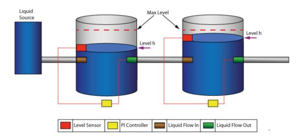
A set of diagrams is created in Enterprise Architect that models the physical aspects of the tanks and the equations (written in the Modelica/MATLAB language) that characterize the flows between the tanks. Once the simulation has been configured and the *Solve button* selected, the output resembles this diagram:
