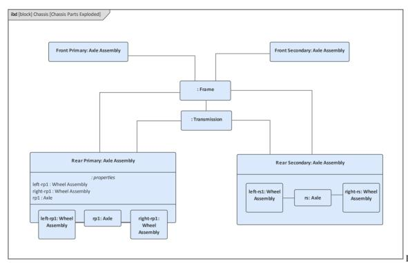
diagram the Rear Primary and Secondary Axle Assemblies have been shown in detail, where each Axle is composed of a right and left wheel assembly, which themselves could be shown as a nested structure comprising the Brake Assembly, which in turn could show the Wheel Cylinder Assemblies.
