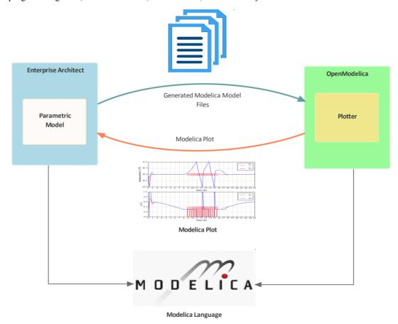
An overview of how it works can best be provided by way of a simplified example. To create a simple visualization of Newton's Second Law - 'The rate of change of momentum is proportional to the force acting and takes place in the direction of that force.' (F = m\*a), an engineer using Enterprise Architect will:
