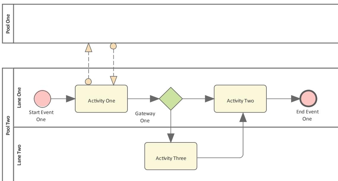
Black Box Collaboration diagram, showing Message Flows that originate from flow objects and target the boundary of the other participant's Pool.
