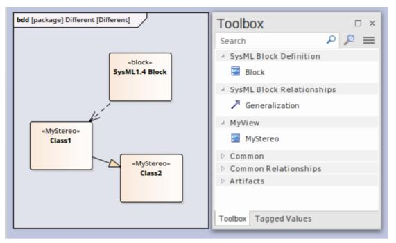
The diagram View makes the elements and connector available from the Toolbox, as shown, and from the Quick Linker.
