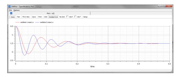
• Mass, light vs heavy: the object with smaller mass will oscillate faster and regulate more quickly
