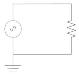
The circuit includes an AC power source, an earth and a resistor, connected to each other by electrical wire.
