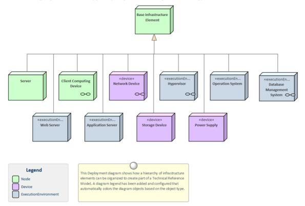
The Technology elements section of the TRM is a hierarchical structure and classifies parts of the infrastructure based on their function as a Physical or Virtual Node, Device or Execution Environment. This allows any type of technology concept, physical or virtual to be modeled including a wide range of infrastructure pieces such as servers, routers, operating systems, hypervisors, database management systems, web servers and more.
