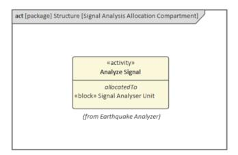
Any element that allows compartments can be configured to hide or show any number of available compartments. The list of compartments is specific to an element and is dynamic, meaning that a compartment will only be visible if the element participates in one or more relationships of the specified type and the relationship is not visible on the containing diagram. The same options can be used to display a range of other structural or semantic aspects of the elements as shown here.
