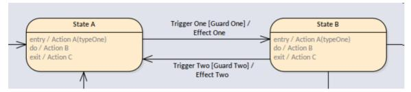
The transitions always originate from one State and target another, including the special case of a self-transition where the origin and the target are one and the same. The lines in the diagram have a label that can display a number of different options: *Trigger*, *Guard* and *Effect*. We will discuss these options in detail because they express important semantics about the transitions, including whether the transition will be executed at all. A transition can be in three conditions:
