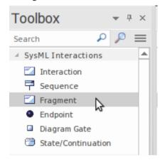
The element placed on the diagram is a generic Fragment and will need to have its operator set. This can be achieved by selecting a value for the type in the Combined Fragment property sheet.
