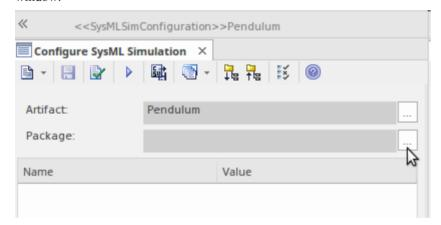
Enterprise Architect will display the Package selection window, and once the Package is selected the 'Configuration' panel will be populated with the Blocks, ConstraintBlocks and Value Types from the model. From this point the values can be entered for various parameters, or data-sets can be defined. The simulation configuration parameters can be entered and the simulation is ready to run.
