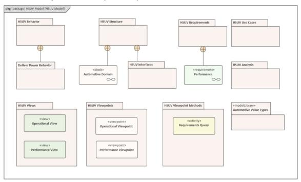
The relationships between the Operational View and the Performance View and the rest of the user model are explicitly expressed using the «import» relationship. The Packages that appear in the diagram are defined and can also be visualized in a hierarchical view using the Browser window.
