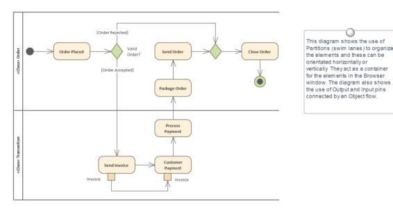
The elements can be given a name and detailed descriptions can be added to the Notes. By connecting the Activities, Decisions and Forks with connectors (Control Flows) a sequence of elements can describe the business process. A process hierarchy can be constructed by nesting Activities in the Browser window and using the child diagram functionality to enable drill down from the value chain level to the lowest level processes.
