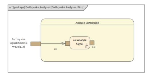
The Parameters and Pins are collectively known as Interaction Points, signifying that they are locations where an element interacts with its environment; they can be selected for inclusion on a diagram by using the multi-purpose Features window.
