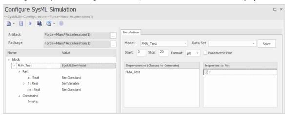
3. Run the Simulation by selecting the Solve button on the window.
