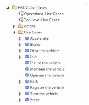
Enterprise Architect also provides a number of helpful and unique tools to assist the Systems Engineer to efficiently describe the Use Cases and define Scenarios that detail the steps representing the interaction between the Actor and the System. Once these have been defined the tool can automatically generate behavioral diagrams directly from the model.
