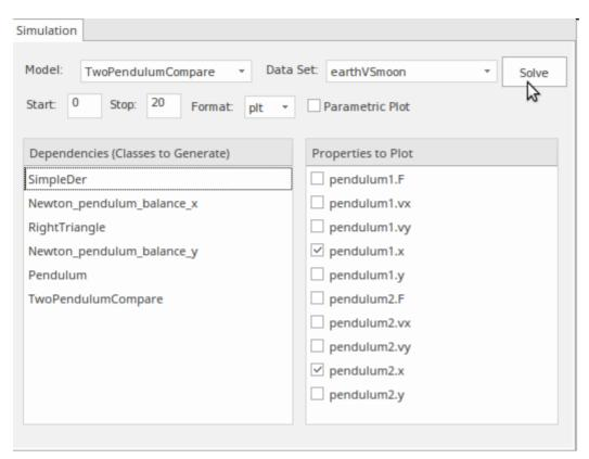
The information in the window is automatically populated from the model that is visible in the Browser window, and the location of the elements - including Value Types, Blocks and Constraint Properties - can be found using the 'Find in Project Browser' option from the context menu. There is also an analogous option to find the selected element in any diagrams in which it appears.
