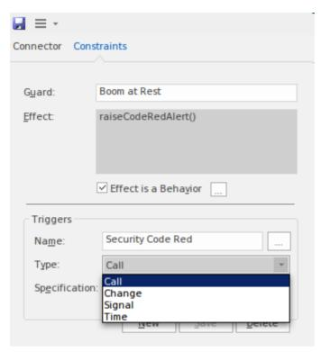
This diagram illustrates the way the Trigger, Guard and Effect are displayed on a diagram. The Effect in this case has been defined as a behavior and has been linked to an Operation defined on the Block.
