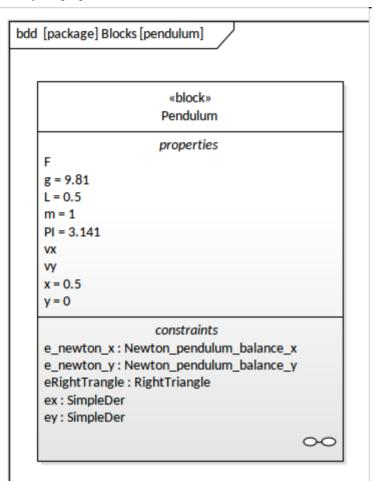
In preparation for defining the equations that define the behavior of the pendulum system, we will define the value types required to ensure the model is precise and check that the simulation parameters are correctly specified. This is done using a Block Definition diagram (bdd), using the Value Type element available from the Diagram Toolbox.
