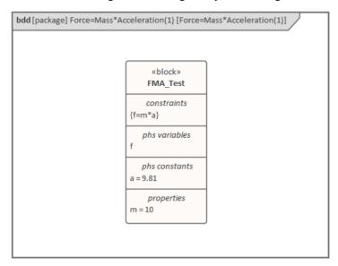
2. Configure the SysMLSim Configuration Artifact (used to define the information needed by OpenModelica).
