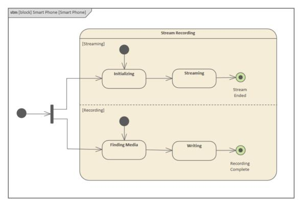
Joins work in an analogous but opposite way to unite incoming transitions from multiple regions. The reverse restriction applies such that the *incoming* transitions cannot have a guard or a trigger defined but an Effect can be defined. The Effects for all incoming transitions must be completed before the outgoing transition can fire.
