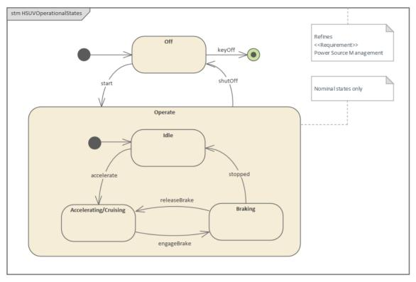
The message in the Sequence diagram Start Vehicle is the trigger that will cause the vehicle to transition from the Off state to the Operate (on) state. Enterprise Architect allows these transitions to be defined in detail.
