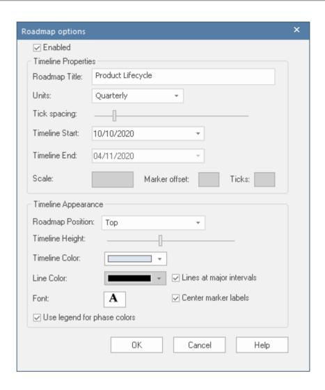
The Diagram Legend can be configured to define the phases in the element's lifetime, to set the specification of the colored bands and more. Roadmap segments can be shown or hidden on individual elements in cases where a particular segment might not apply to one or more of the elements on the diagram.
