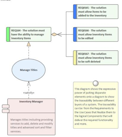
Use Case diagrams can be used to show how the Use Case are related to other elements in the system, including up-stream elements such as Requirements and down-stream elements such as Components.
