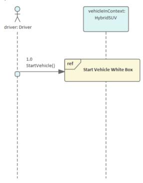
This exchange of messages and signals, and the consequent behaviors, can be represented on a Sequence diagram that shows the time-sequenced messages and signals between Block instances that participate in a specific interaction.
