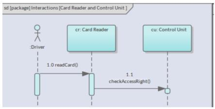
The sender is effectively calling or activating some behavior provided by the receiving lifeline. Enterprise Architect provides useful mechanisms to utilize behaviors already defined in the form of operations. This illustration shows the properties of an existing message, which the modeler is able to select from a drop down list of previously defined operations. Alternatively, the modeler can define a new operation by selecting the Operations button.
