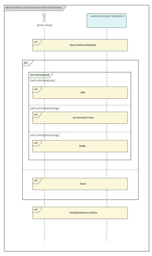
This diagram uses a type of element called a Reference, which acts as a place holder for another Sequence Diagram. Enterprise Architect conveniently allows these diagrams to be opened by double-clicking on the 'ref' element in the diagram.
