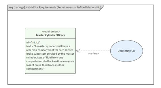
In these two diagrams the modeler has used the <<refine>> relationship to indicate that the *Decelerate Car* Use Case refines or adds additional explanation to clarify the Requirement *Master Cylinder Efficacy*. This provides a mechanism to trace implementation level components that are connected to the Use Case back up to the Requirement and ultimately to the Stakeholder.
