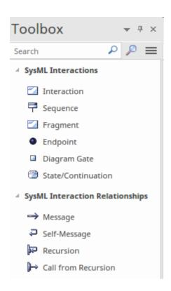
Elements can be added to the diagram by dragging-and-dropping them from the Browser or from the Toolbox onto the diagram canvas. The typical process is to reuse existing elements such as Blocks, which have behaviors in the form of operations that can be selected as the basis for the messages that are exchanged between lifelines. The elements can be added to the diagram as a link but more typically they are added as a lifeline.
