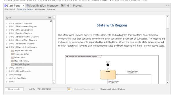
This image shows a diagram that has been created from the *State with Regions* pattern, which has been simply injected into the model and acts as a starting point for the modeler. The modeler can tailor the diagram by replacing the names of States and Transitions and adding or deleting regions as required.
