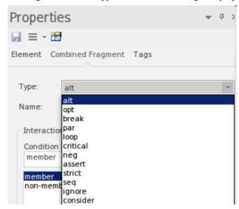
This will change the fragment to the appropriate type and allow, for example with the *alt* type, to set any number of alternative conditions that will determine which message will be fired.
