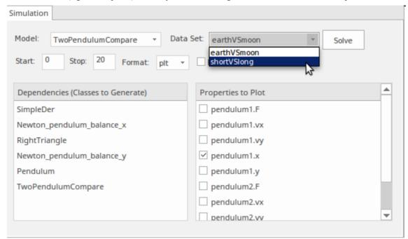
Any number of data sets can be defined and can be added to the appropriate Block in the 'Configuration' (left-hand) panel of the Simulation window. These are available as nodes under each Block and there is an option to view and edit the data values in a window by using the Browse [...] button on the datasets row.
