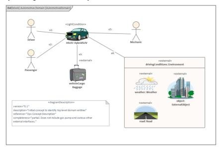
Enterprise Architect also allows the conventional symbols of the SysML to be replaced by more appealing and meaningful images that assist in the acceptance of the diagram by non-technical audiences.
