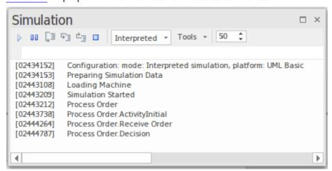
Note the text entry box just underneath the toolbar. This is the Console input area - here you can type simple JavaScript commands such as: this.count = 4; to dynamically change a Simulation variable named 'count' to 4. In this way you can dynamically influence simulation at run-time.
