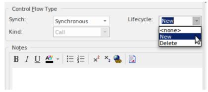
Setting this property has the effect of moving the targeted Block to a position lower in the diagram, signifying that the Block Instance would not be created until this point in the overall time sequence of the diagram. The message line style is also altered to a dashed line with an open arrow-head to reflect that it is a *Create* message. Other aspects of the semantics and effect of this message are unchanged.
