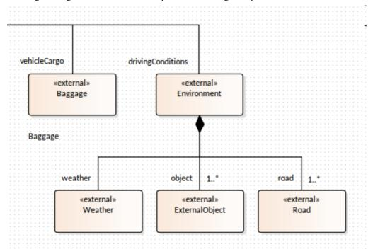
This change of element appearance can be applied at a (default) global level or at a diagram specific level allowing alternative presentations to be created for different audiences.
