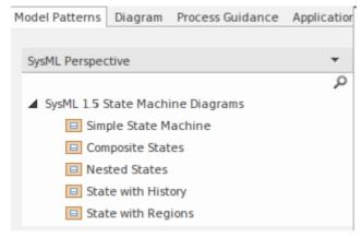
The pattern can be used to create a number of different StateMachines; in this example we create a simple (single region) diagram that has all the appropriate detail added to the States and the Transitions. A modeler can create this diagram in the appropriate location in the repository and then edit the States and Transitions and diagram to make it suit their own modeling context. The initial StateMachine diagram created from the pattern will resemble this:
