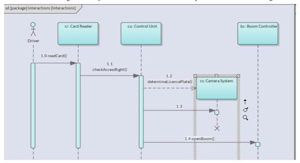
When a Sequence diagram is representing a software system that has bounded memory available, the destruction of the targeted instance will result in allocated memory being returned to the memory pool. In systems engineering there can be a variety of other pay-offs from managing the lifetime of electro-mechanical objects, such as power consumption, over-heating, availability, or even risks such as security.
