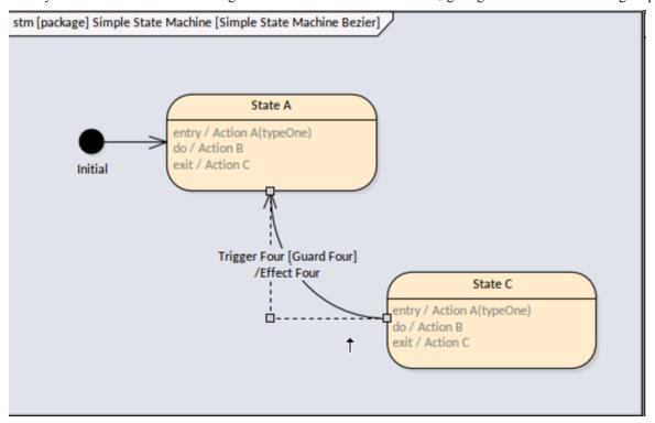
The shape of the curve can be altered by dragging the construction point to a new location. Any one of a number of line styles can be used, providing the modeler with a toolkit of options for diagram presentation. This context menu can be selected and the line style set for each connector individually. The color and thickness of the line can also be set from the Layout ribbon.
