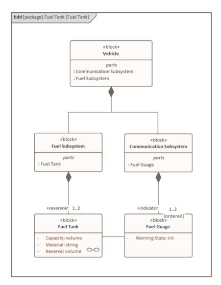
In the Fuel Tank diagram the car is modeled as a classifier (Block) level, where the model is describing a generic vehicle and representing the fact that a vehicle could have one, or a maximum of two, fuel tanks. This Fuel Tank Instances diagram, however, describes a particular vehicle that has two fuel tanks that have different capacities and reserve volumes.
