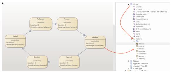
When you browse for the diagram in the 'State Transition Recorder' dialog, the hierarchy shows only the root Package, parent Class and child SubMachine and diagram; no other model components are listed.
