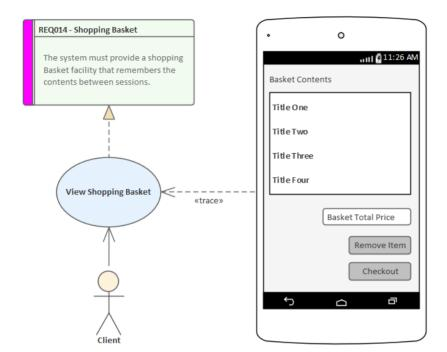
This diagram shows traceability from a Requirement to a Use Case and the User Interface for a web application running on an Android Phone. The controls are elements that can be linked to information items that can model the source of the data.
