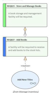
This diagram shows a Use Case that realizes a requirement. The realized requirement is part of a hierarchy of requirements expressed with the Aggregation relationship. The Use Case has an annotation under the element indicating its package location in the Browser window.
