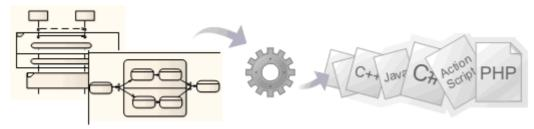
Enterprise Architect's multi-featured system engineering capability can be used to generate code for software, system and hardware description languages directly from behavioral models, such as StateMachine, Sequence (Interaction) and Activity diagrams. The supported languages include C(OO), C++, C#, Java, VB.Net, VHDL, Verilog and SystemC.
