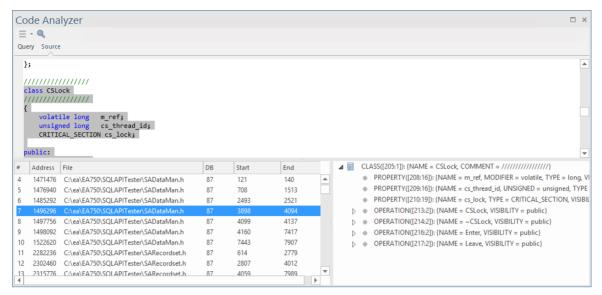
Selecting a detail item in the lower-right panel, results in narrowing the selection within the source code, as shown here.
