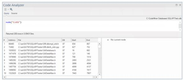
By selecting a result in the lower-left panel, the 'Source' tab is activated and displays the source code corresponding to the selected node. Details for that class node are displayed in the lower-right panel.
