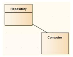
These Classes are instantiated as Objects in an Object diagram. There are two instances of Computer in this model, demonstrating the usefulness of Object diagrams in considering the relationships and interactions Classes might have in practice.
