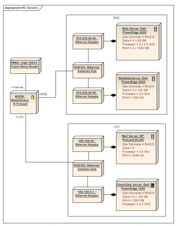
Deployment diagrams are ideal for applying alternative images to depict the objects that the elements represent. Such images can be substituted for the elements in the diagram, as shown here:
