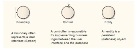
You apply a new appearance or shape by associating the stereotype with either a metafile (image file) and fill, border and text colors, or a Shape Script that defines the shape, dimensions and text of the object.
