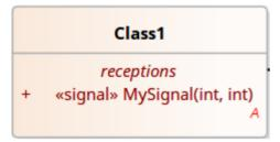
A Reception cannot be created without a Signal element, which either already exists or is created as a step in creating the Reception. The name of the Reception is drawn from the name of the Signal element, and the attributes of the Signal define the parameters of the Reception. Any changes to the Signal are reflected in the Reception, and vice versa.
