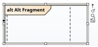
To move a Combined Fragment *independently* of its contents, make sure the 'move freely' element icon is visible; if it is not shown, click on the 'move contents' icon and drag the element border.
