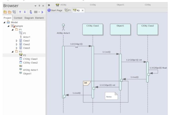
This diagram is not damaged when round-tripped through Version Control, because all the Lifelines are objects and these objects reside in the same Package as the Sequence diagram.
