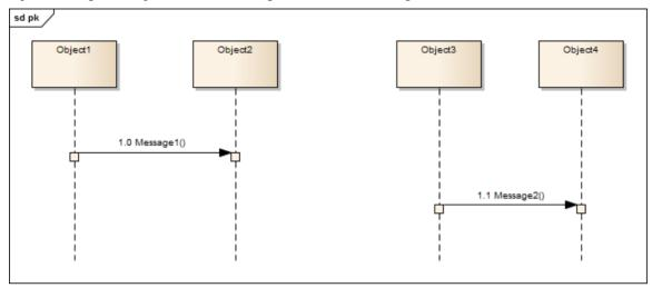
In the diagram, Message 1 is earlier than Message 2. However, in a complex diagram, or when representing finely timed operations or parallel processing, this might not be apparent. You can reinforce the sequence using a 'General Ordering' arrow.
