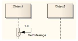
A Self-Message reflects a new process or method invoked within the calling lifeline's operation. It is a specification of a Message, typically in a Sequence diagram.
