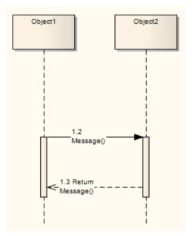
Sequence diagrams depict workflow or activity over time using Messages passed from element to element. In the software model. These Messages correspond to Class operations and behavior. When you display a Sequence diagram, the Diagram Toolbox automatically switches to the 'Interaction' pages of the Diagram Toolbox, containing the 'Message' icon.
