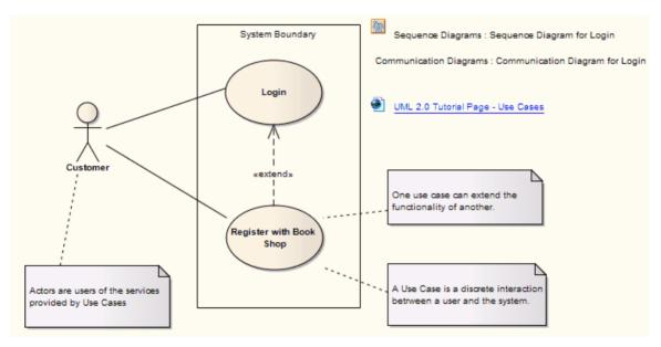
If extending a Use Case, you can specify the points of extension with Use Case Extension Points. To display the attributes, operations or constraints of a Use Case on a diagram, use Rectangle Notation.
