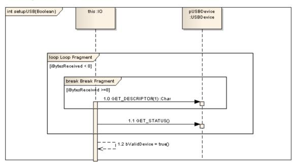
An Interaction element in Enterprise Architect is treated as a behavior of the classifier it is encapsulated within. It can have parameters and return types, which are modeled using the 'Behavior' tab of the Interaction element's 'Properties' dialog. The element is interpreted as a method of the containing Class in the generated code (see the *Generate Code From Behavioral Model* topic).
