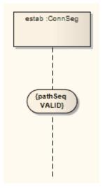
When a State Invariant is moved near to a Lifeline, it snaps to the center. If the sequence object is dragged left or right, the State Invariant moves with it.
