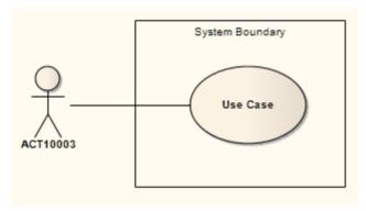
You can also define a Use Case as the classifier of a System Boundary element, to link the elements enclosed in the System Boundary (such as parts of an Activity diagram) to their representation in a logical Use Case.
